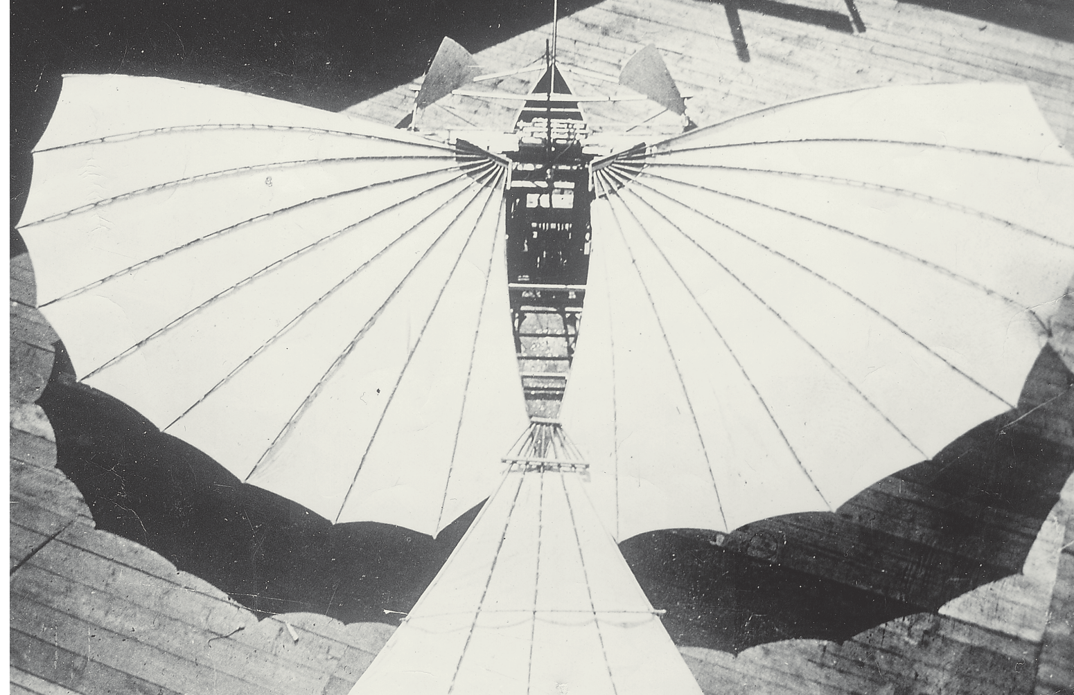
An original 1901 overhead view of Gustave Whitehead's powered monoplane. In 1986, by underexposing prints during the construction of the first reproduction, we were able to see where the ground engine was installed (pushrods and their shadow show in cockpit-area floorboards behind the mast). What looks to be the top of his generator is behind the ground engine in the dark, shadowed region. No detail of its design can be determined. Numerous persons, including Whitehead's associates, recalled seeing the generator working the "steam-type" engine while on a test block and when the airframe was making short hops along the dirt roads near Whitehead's shop before and after the claimed August 14, 1901, events.
