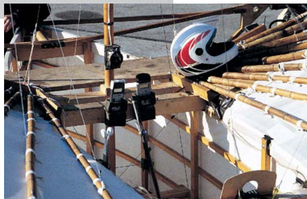
A close view of the cockpit and wing-root region of the German reproduction. The forward ends of bamboo-cane ribs swivel on bolts that are fastened through the rib tray.
